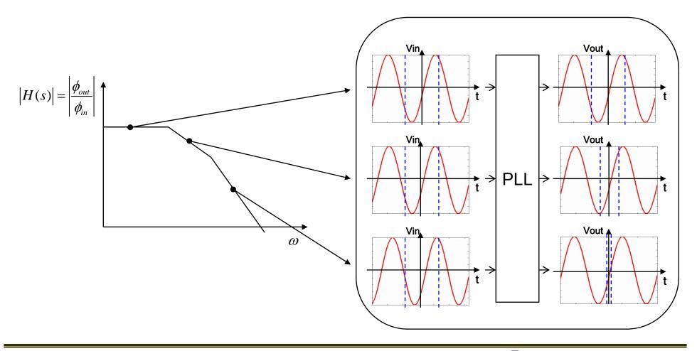
$$H(s) = \frac{\phi_{out}}{\phi_{in}} = \frac{K_{PD}K_{VCO}\omega_p}{s^2 + \omega_p s + K_{PD}K_{VCO}\omega_p}$$
